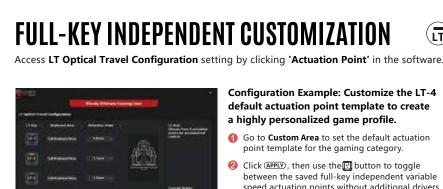
between the saved full-key independent variable speed actuation points without additional drivers. 3 Click on 'Advanced Setting' to access the actuation point editing platform and adjust the speed of both full-key and independent key actuation
